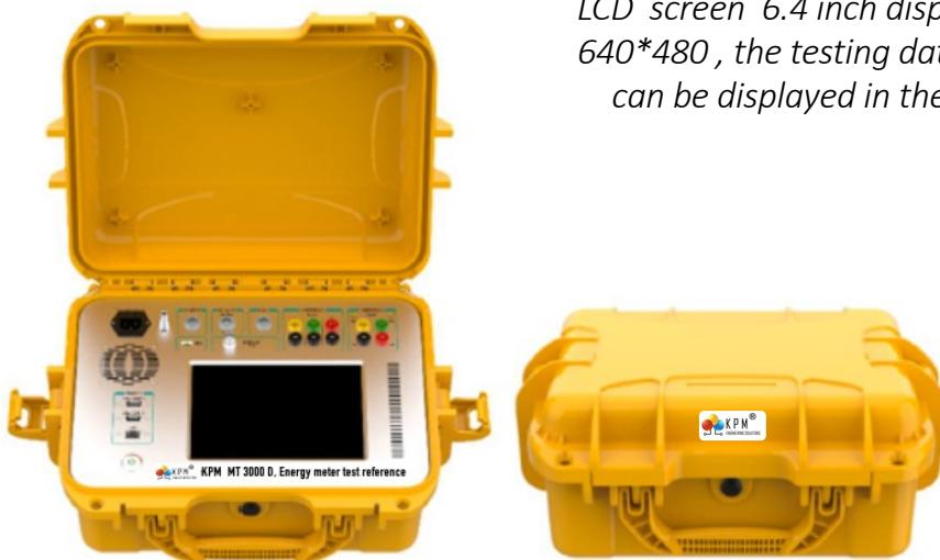
**MT 3000D is a portable Energy Meter Test Reference with 0.02% & 0.05% Accuracy**
