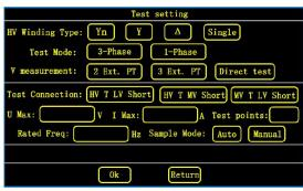
Transformer Short-circuit impedance test setting interface
