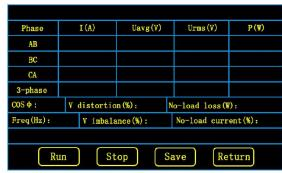
Transformer No-load test running interface
