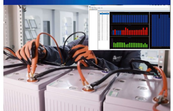
Using probes to touch battery poles to proceed test
