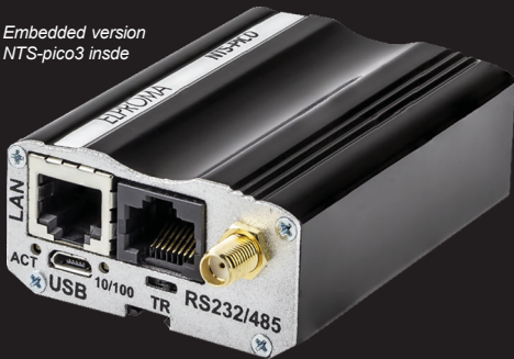
The LAN1 is hosted on embedded ver. of well known NTS-pico3. The special embedded version of NTS-pico3 inside ANT version controls GNSS, MANAGEMENT, PoE and autonomous LAN2-3. The NTS-pico3-ANT product is all-in-one assembled inside dome bullet class industrial housing and it is powered PoE (LAN1).
