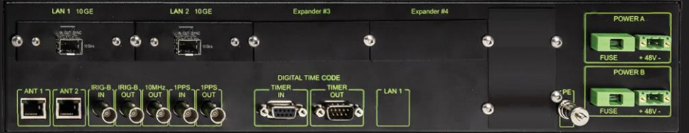
TELECOM-3 PRTC-A 2x10GbE, 48VDC SW-stamping NTP-Server w/ PTPd support
